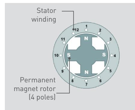
The rotor speed of rotation is characterised by the following equation:  $N = N_s = 120 \times (f) / \text{No. of poles per phase}$ .
