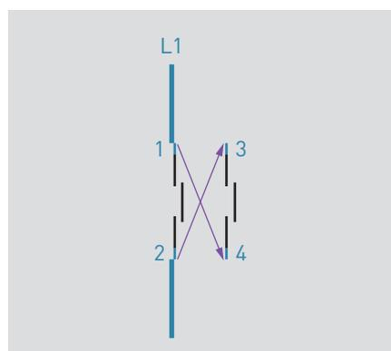
It is advisable to connect contacts in parallel by crossing over the connections, so as to divide the current equally in each pole.
