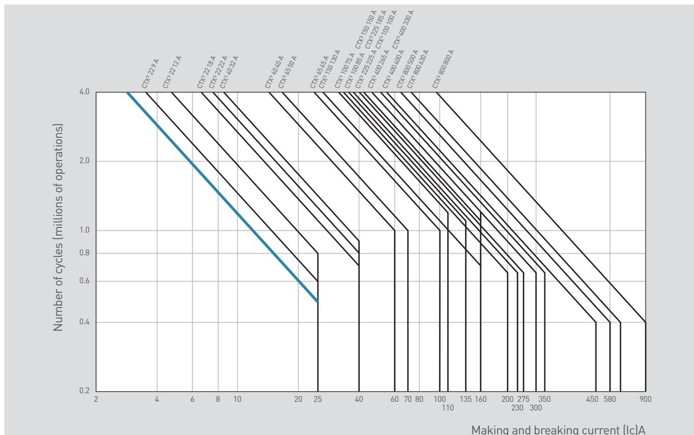
Example: For an AC-1 operating current of 50 A and endurance of 2 million operations for an external ambient temperature below 40°C, you should select a 65 A CTX<sup>3</sup>.
