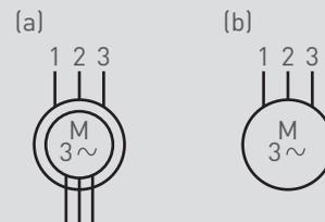
Electrical symbols for wound rotor (a) and squirrel cage (b) asynchronous motors
