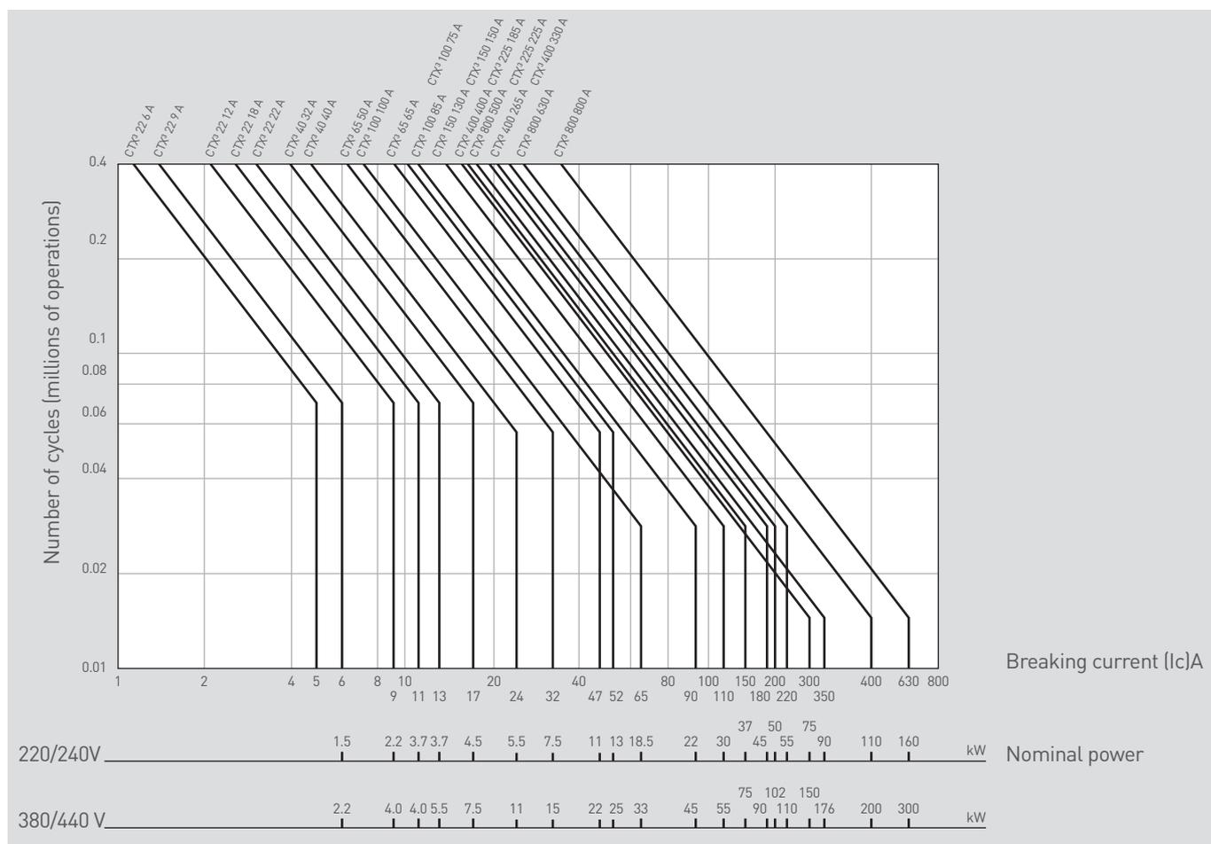
Example:  $I_c = 6 \times I_e = 66 \text{ A}$  for a 5.5 kW motor,  $U_e = 400 \text{ V}$   $I_e = 11 \text{ A}$ . For endurance of 200,000 operations, you should select a 22 A contactor.
