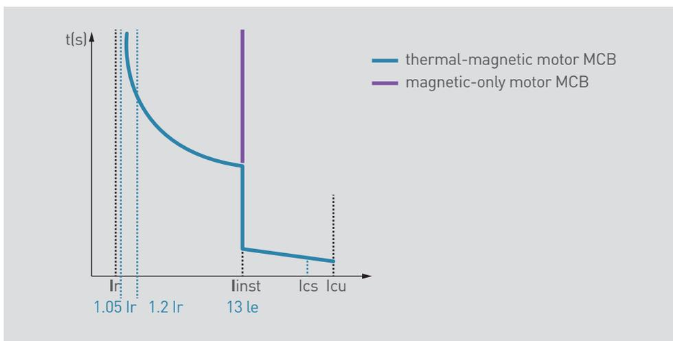
The circuit breaker should not trip for  $I \leq$  or  $= 1.05 I_r$  (setting current), in compliance with the requirements of standard IEC 60947-4-1. Above  $I_r$ , in the event of a thermal overload, the circuit breaker trips in a time inversely proportional to the current flowing across it.
