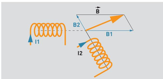
In the case of the three-phase motor, the three coils are positioned in the stator at 120° from one another, which creates three magnetic fields. Given the nature of the current on the three-phase supply, the three fields are phase-shifted.
