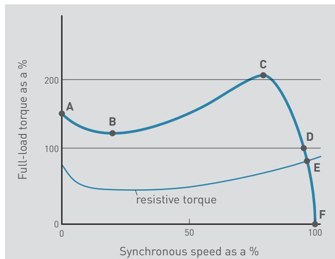
**A: Starting torque or breakaway torque:** This is the value of the torque delivered by the motor when it is powered up, at the point when the rotor starts to move. It can only be applied for a few fractions of a second and it is directly proportional to the power supply voltage. It is the same as nominal torque for synchronous motors. It is therefore important to check the motor operating voltage range in these starting conditions and particularly to take account of the voltage drop.
