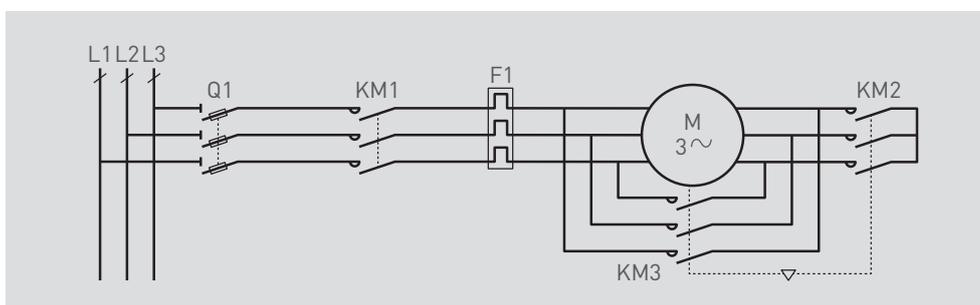
There is a method consisting of inserting a resistor before opening the star contactor to prevent the occurrence of transient phenomena associated with the sudden power cut. However, this process is rather more complicated and expensive to implement.
