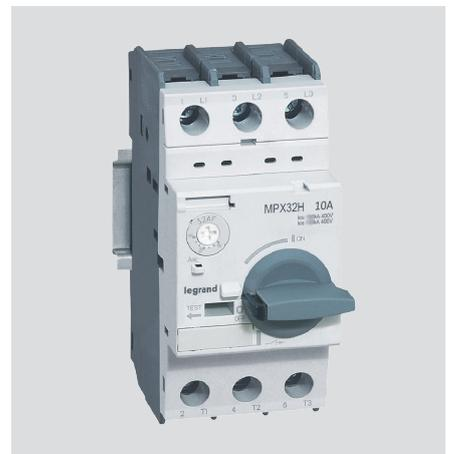
The motor MCB can be “magnetic only” type, in other words without a thermal protection component. In this case, it only offers protection in the event of a short-circuit. It is often used for smoke control applications, in which the motor should continue to run, including when there is a fault associated with an overload. For certain starting modes using contactors, with thermal protection provided by a thermal relay, a “magnetic only” type circuit breaker is sufficient.
