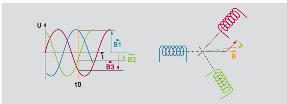
When supplied in this way, the stator generates a magnetic field, called a **stator field**, rotating at a speed called **synchronous** ( $N_s$ ). The rotation frequency of this field is linked to the frequency of the mains supply and the number of pairs of poles in the winding.  $N_s = 60 \times F / P$  (F frequency, P no. of poles), in number of revolutions per minute (RPM).
