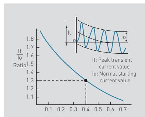
For a power factor on starting of 0.4, the inrush current reaches 1.3 times the normal starting peak current ( $7 \times I_n \times \text{root of } 2$ ). If the motor restarts before the end of its rotation, this current surge can be twice as high. In this case, it can reach 2.6 times the nominal starting current, due to the residual current in the motor.
