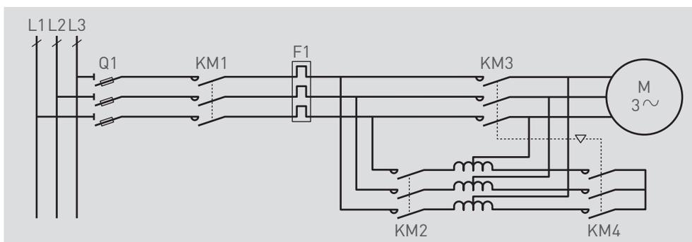
Depending on each starting current connection and ratio, the switching current varies from 1 to 5 x  $I_n$ . The torque delivered varies in proportion with the starting current.
