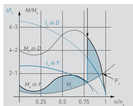
Sequence: when the speed of motor rotation stabilises (equilibrium between motor torque and resistive torque), at a speed of approximately 85% of nominal speed, the windings are then connected in a delta configuration and the motor regains its natural operating characteristics.
