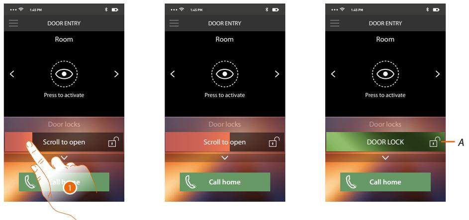
A. When it becomes green the door lock has been activated. If it remains red, the command has not been performed correctly.
