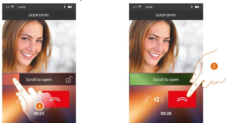
4. You can also open the door lock of the Entrance Panel from which the call comes, by dragging the switch. When it becomes green the door lock has been activated. If it remains red, the command has not been performed correctly.
