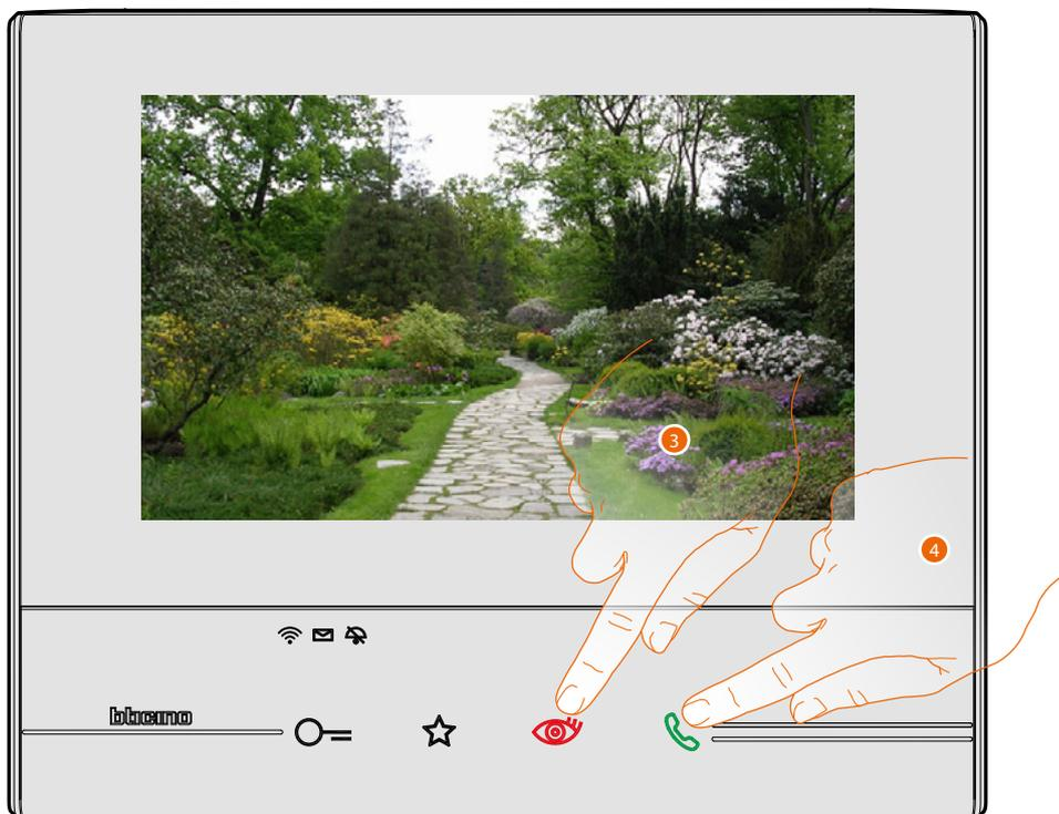
3. Touch to display another camera (scrolling). When switching from one camera to the next, the key lights up.
