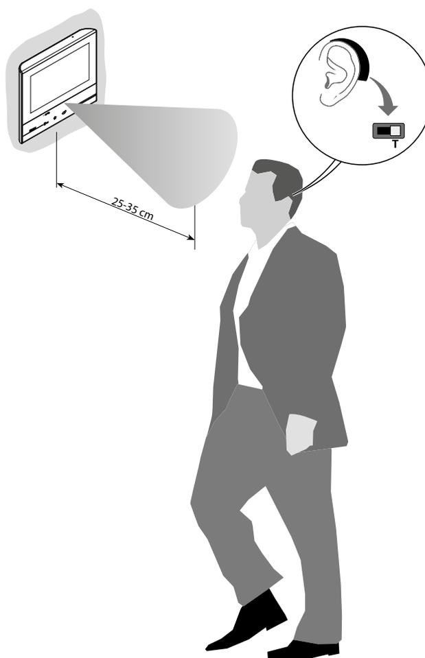
To ensure correct magnetic coupling between the IU and the acoustic device, we recommend a position in front of the device, at a distance of 25-35cm. It is reminded that the presence of metal and background noise generated by electric/electronic devices (e.g. computer) may compromise the performance and the quality of the coupling device.
