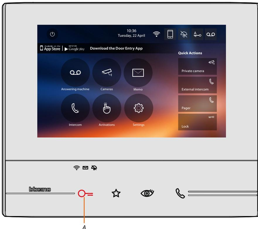
A. LED flashing = door lock open.
