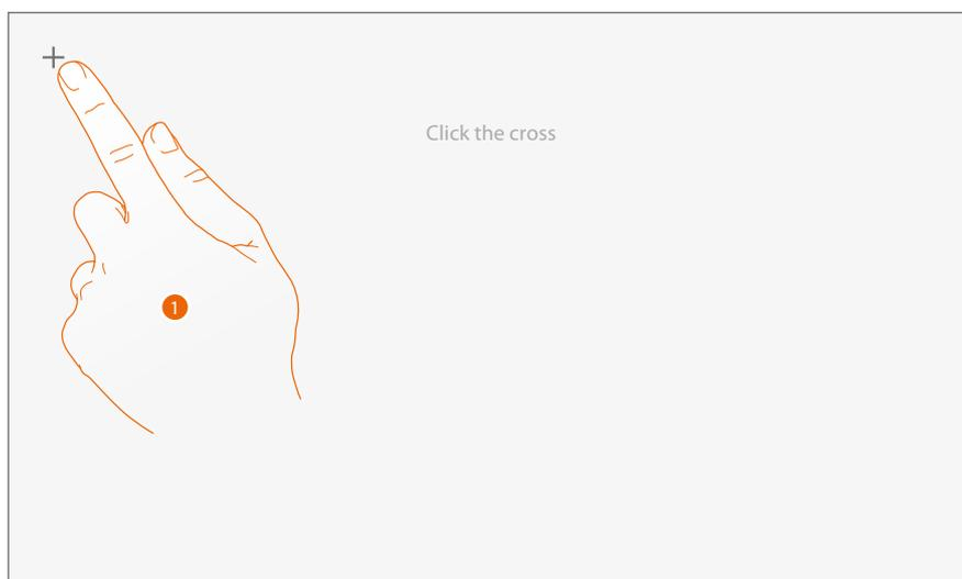
1. Touch the "cross" symbol on the display as it moves to all 5 positions. At the end, the **OK** icons appears at the corners of the display. Touch it to complete the calibration procedure.
