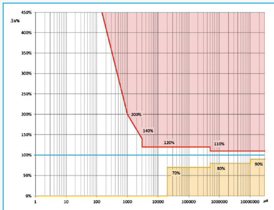
ITIC curve: the area in WHITE represents all of the combinations of variations in supply voltage and duration, in which the electronic device does not experience any changes in operation.
