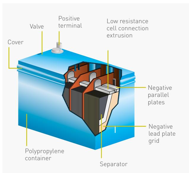
VRLA batteries are sealed hermetically, do not require any maintenance work, and have an internal gas recombination feature. In addition to ensuring a longer operating life, this feature also allows the UPS to be installed in rooms where people regularly linger.
