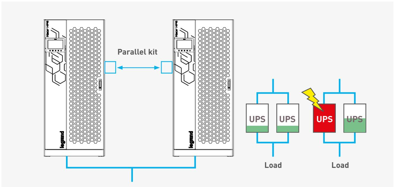
One unusual feature of the parallel architecture is the synchronization of the bypasses: the parallel architecture must also take into account the synchronization of the static bypasses of each UPS along with any external manual bypass.
