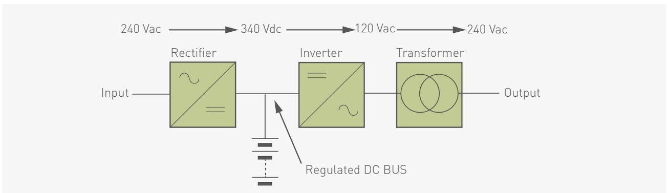
We should stress that this transformer does not necessarily guarantee galvanic isolation between the input and output; in fact, the input neutral is directly connected to the output neutral in the configurations where the ability to switch to bypass is required.
