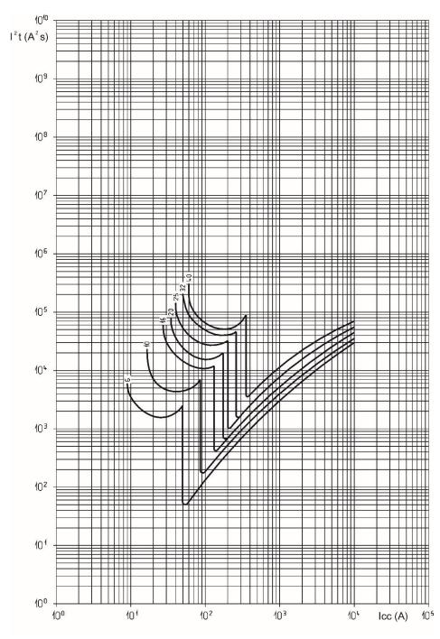
$\label{eq:lcc} \begin{array}{l} Icc = prospective \ short-circuit \ symmetrical \ current \ (rms \ value \ in \ A) \\ I^2t = Iimited \ thermal \ stress \ (in \ A \ s)^2 \end{array}$
