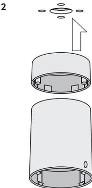
**EN** Secure the mounting box to the extender using the supplied fixings. Then, secure the mounting box to the ceiling using the holes cut.
