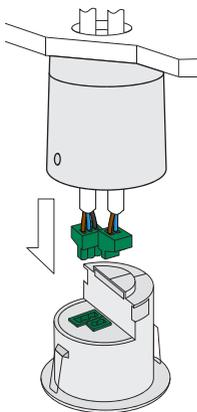
**EN** Wire in plug/s, using wiring diagram on page 2 of the installation guide. Pass the wires through the mounting box and connect the plug/s to the detector.
