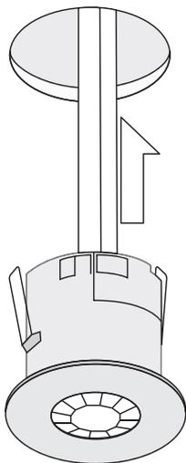
**EN** Bend the springs up and push detector through hole in ceiling. When fully inserted the springs snap back to hold the device in place.
