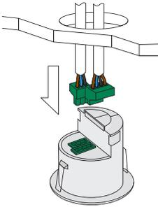
**EN** Wire in plug/s, using wiring diagram on page 2 as a guide. Connect the plug/s to the detector.
