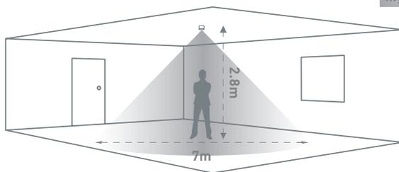
Switched Load and DALI dimming | Switched Load und DALI-Dimmen | Carga conmutada y atenuación DALI | Carga conmutada e escurecimento DALI | Charge commutée et gradation DALI | Carico conmutato e dimmerazione DALI | Geschakelde belasting en DALI-dimmen
