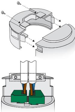
**EN** Continue tightening the screws until the clamp bar snaps out and is tightly engaged against the cable/s. The cable clamp must clamp the outer sheath only.
