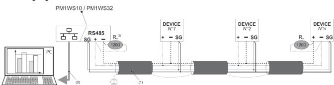
(1) RS485: Prescribed use of Cable Belden 9842, Belden 3106A (or equivalent) for a maximum length of 1000 m, or Category 6 cable (FTP or UTP) for a maximum length of 50 m;
