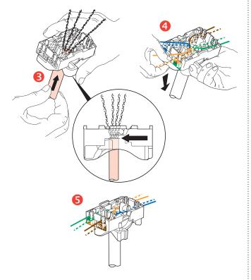
Spreading the cables ensures that a pair-breakage distance of 13 mm is kept between each pair.
