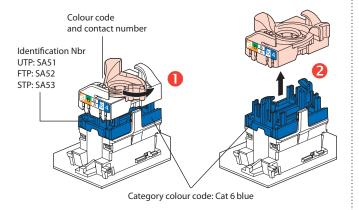
This system allows you to spread pairs before fitting them onto the connector.
