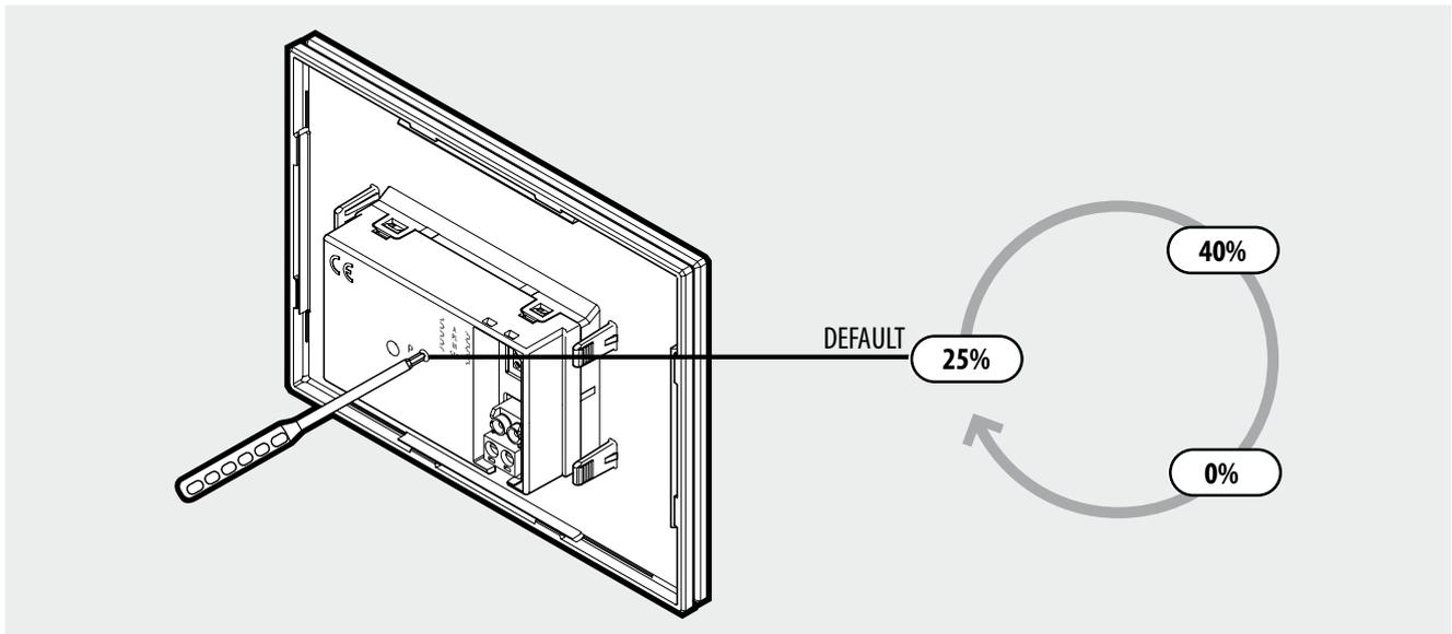
If you have chosen to illuminate the buttons when they are pressed (status return), the brightness level depends on the setting of the LEDs, as indicated below:
