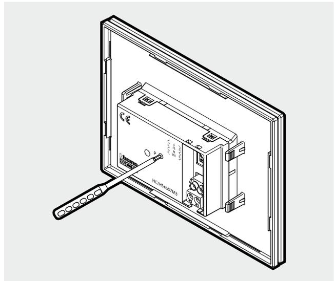
**NOTE:** Use only the screwdriver supplied to operate the P button for programming and LED brightness adjustment.
