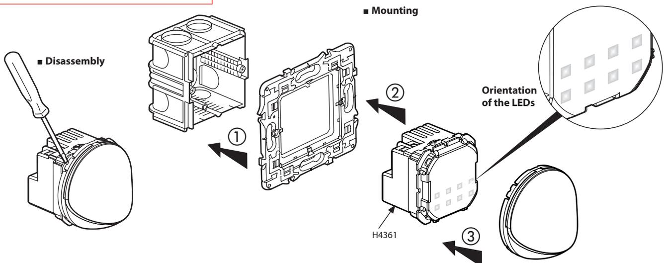
**Note:** Use the same principle for mounting the rotating lamp 360° (H4360)
