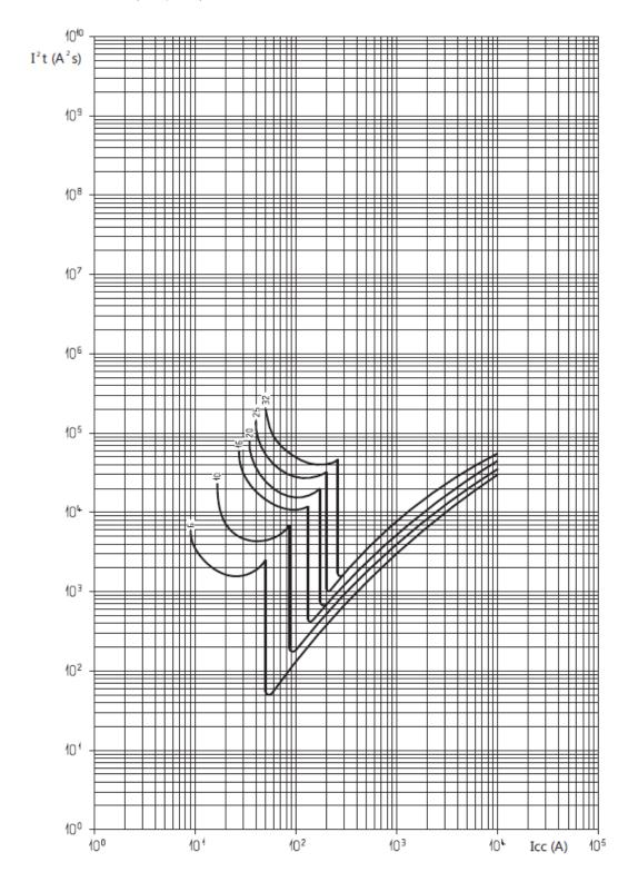
. Icc = Square value of symmetric component of the short circuit current (kA).
