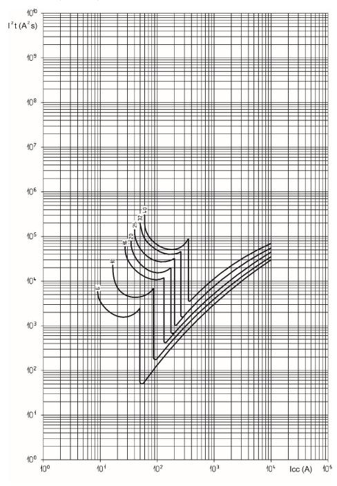
lcc = prospective short-circuit symmetrical current (rms value in A)  $l^2t$  = limited thermal stress (in A s)  $\!^2$
