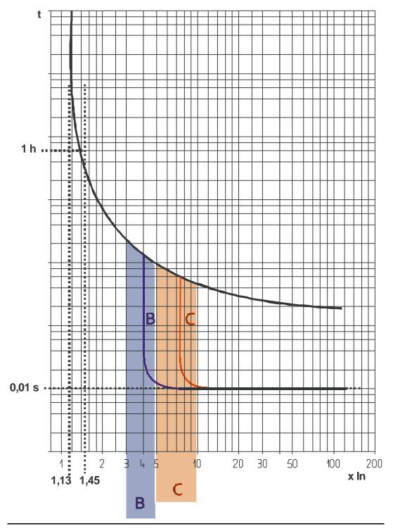
Thermal tripping at ambient temperature = 30°C In = circuit breaker rated current
