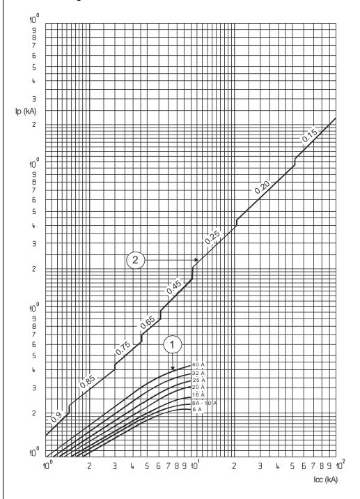
lcc = Prospective short-circuit symmetrical current (rms value in kA) lp = Maximum peak value (in kA) 1 = Short-circuit rms currents (max. peak) 2 = Unlimited peak currents (max.), corresponding to power factors shown above (0.15 to 0.9)
