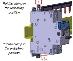
Pull the device downward in order to release it completely from the prongs of the busbar
