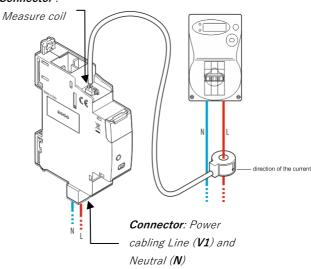
Wire the Smart load shedder after a circuit breaker. The connection between the smart shedder and the current transformer is made via a locking connector.
