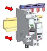
2. Unscrew the terminals and pull the device forward in order to release it from the DIN rail
