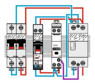
. Control of a three lines standard contactor (>20A):
