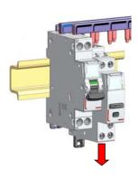
3. Pull the device downward in order to completely release it from the prongs of the busbar
