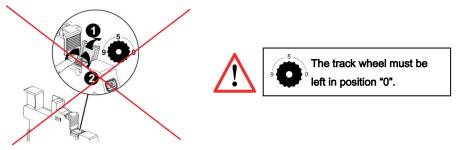
. It is not necessary to address the EMS BTDIN modules. The track wheel must be left in default position "0".
