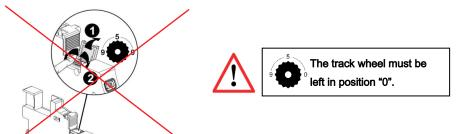
. It is not necessary to address the EMS BTDIN modules. The track wheel must be left in default position "0".
