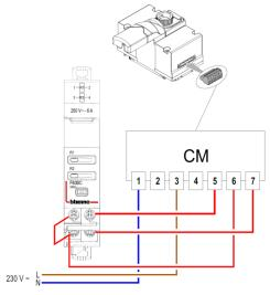
. Association with Motor Driven Control module MEGABREAK up to 6300 A (cat. nos M8MT024C/048C/110C/230C/415/480) with ON/OFF separated commands.
