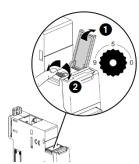
. Marked from 0 to 9 in order to locally define the Modbus address to EMS BTDIN modules In this system the Modbus address of an EMS BTDIN module device or group of modules (several functions) is obtained considering the address of the interface Modbus/EMS BTDIN Interface as tenth and the address of a device or group of function as unit (e.g. Interface address 1 = 10 → address of module n°5 = Modbus address
