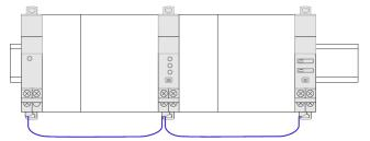
**Implementing:** with this configuration, the plastic protection cover of the backside communication ports on the EMS BTDIN module must be keep on.
