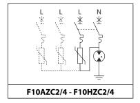
Surge protective devices with L/N-PE and L-N protection modes (common and differential protection modes)
