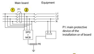
This SPDs can be implemented on upstream side of P1  $\bigcirc$  or downstream side  $\bigcirc$ .
