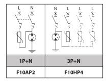
Surge protective devices with L/N-PE and L-N protection modes (common and differential protection modes)
