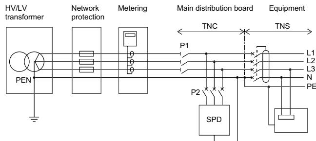
P1: main protective device of the installation
