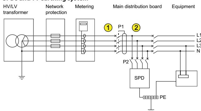
P1: main protective device of the installation
