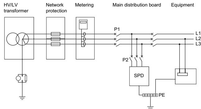
P1: main protective device of the installation
