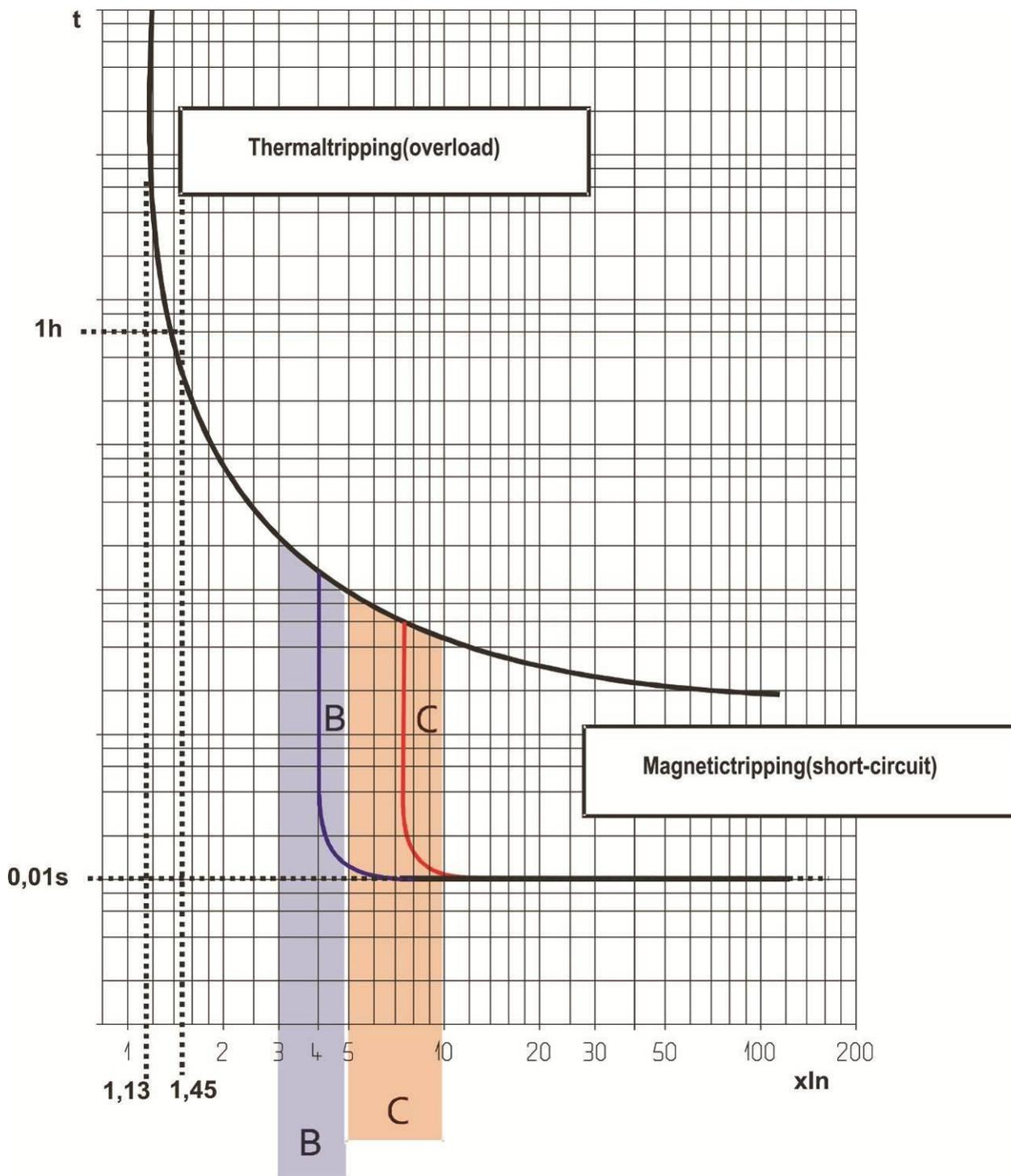
Thermal tripping at ambient temperature = 30°C
