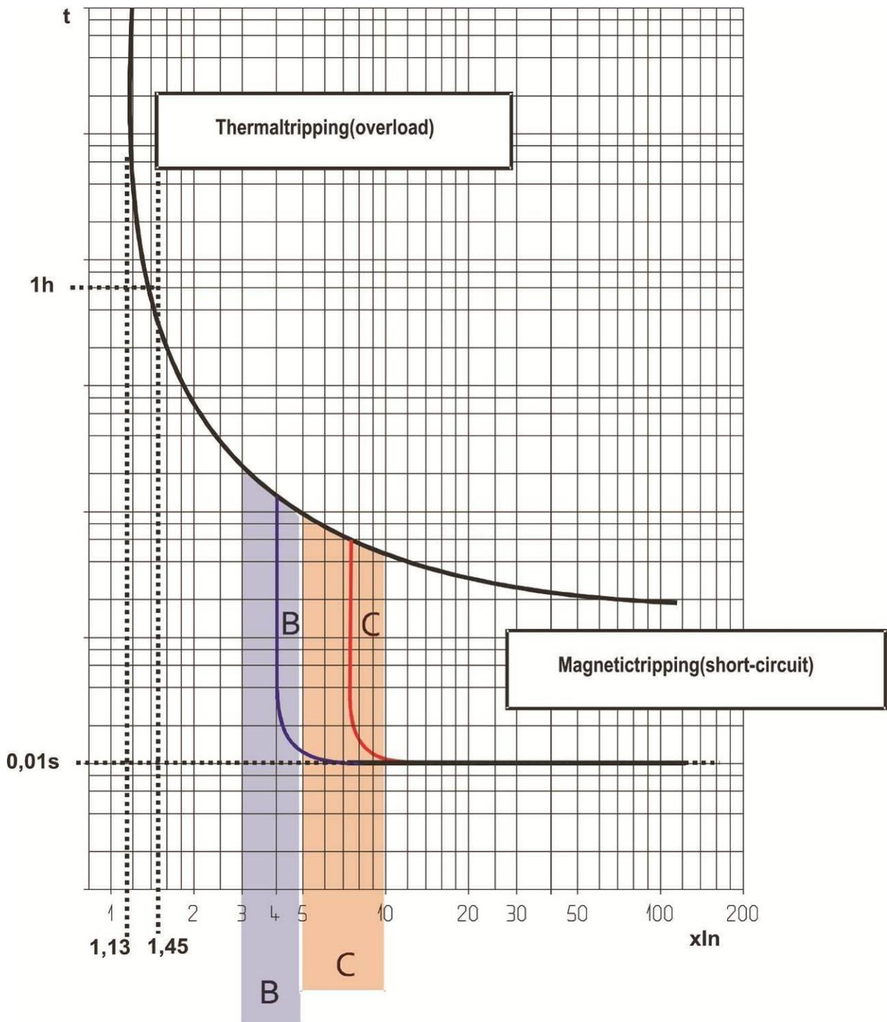
Thermal tripping at ambient temperature = 30°C
