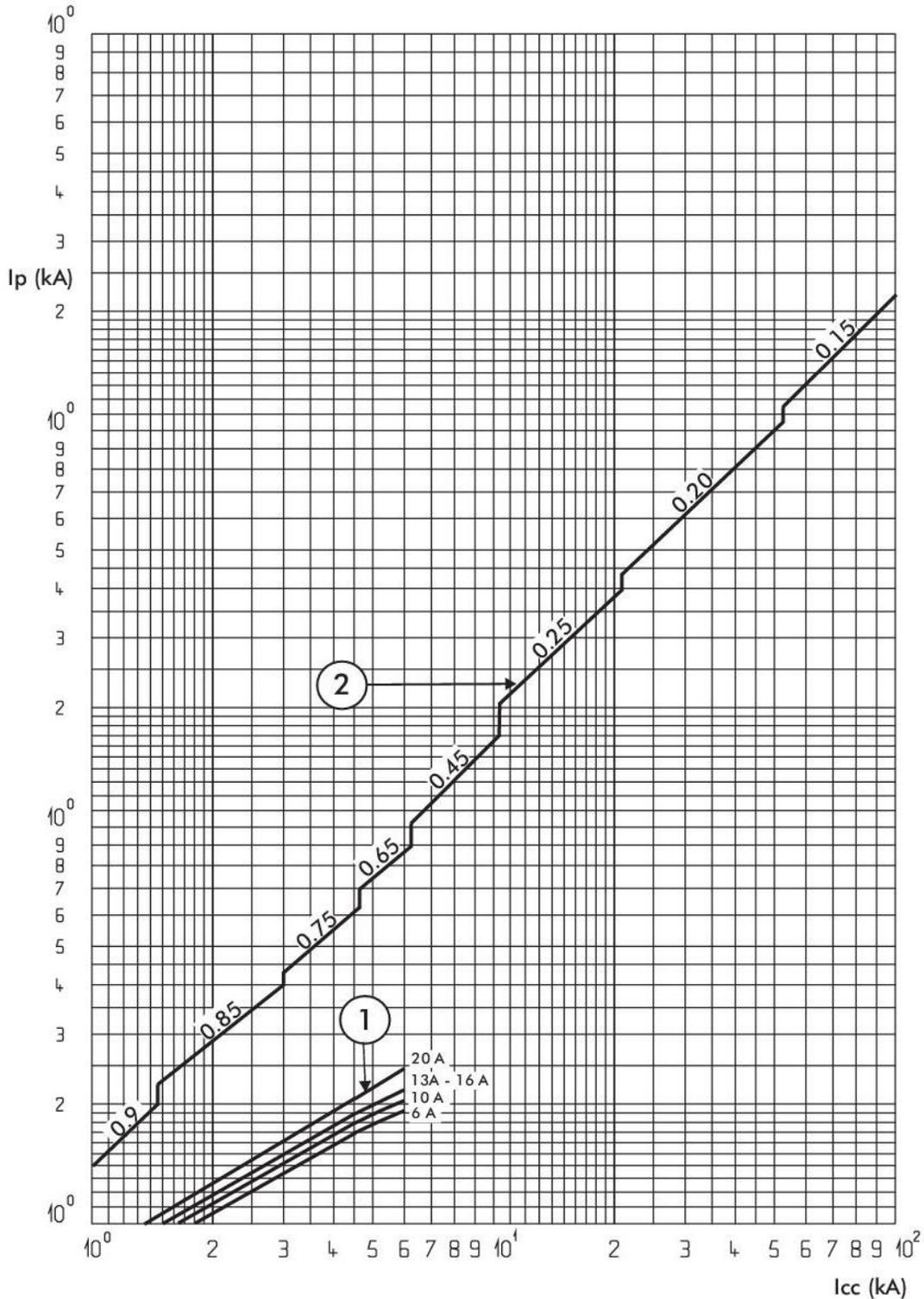
$I_{cc}$  = Prospective short-circuit symmetrical current (rms value in kA)
