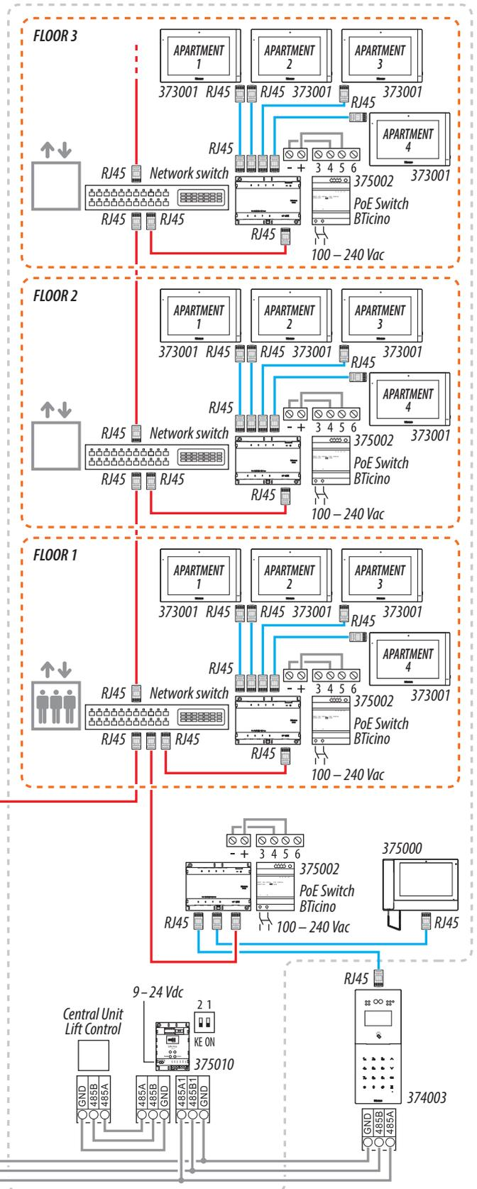
**Attention:** do not directly connect PoE ports to an unsuitable network interface, such as a device powered by a different voltage. Connect the UP LINK port to a suitable port, never to a PoE port.
