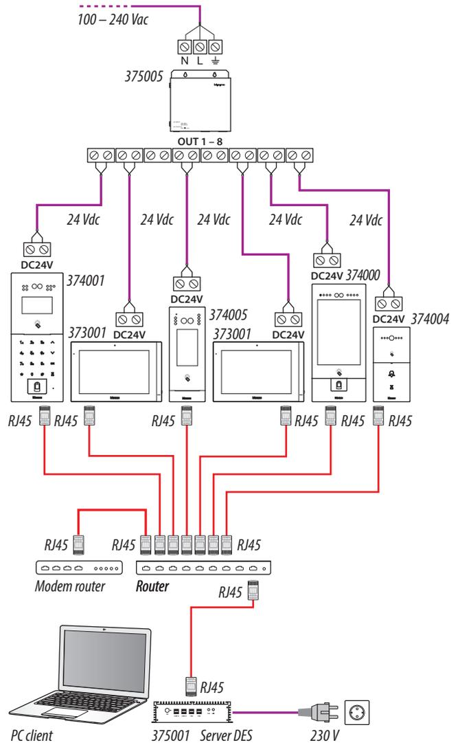
**Attention:** do not directly connect PoE ports to an unsuitable network interface, such as a device powered by a different voltage. Connect the UP LINK port to a suitable port, never to a PoE port.
