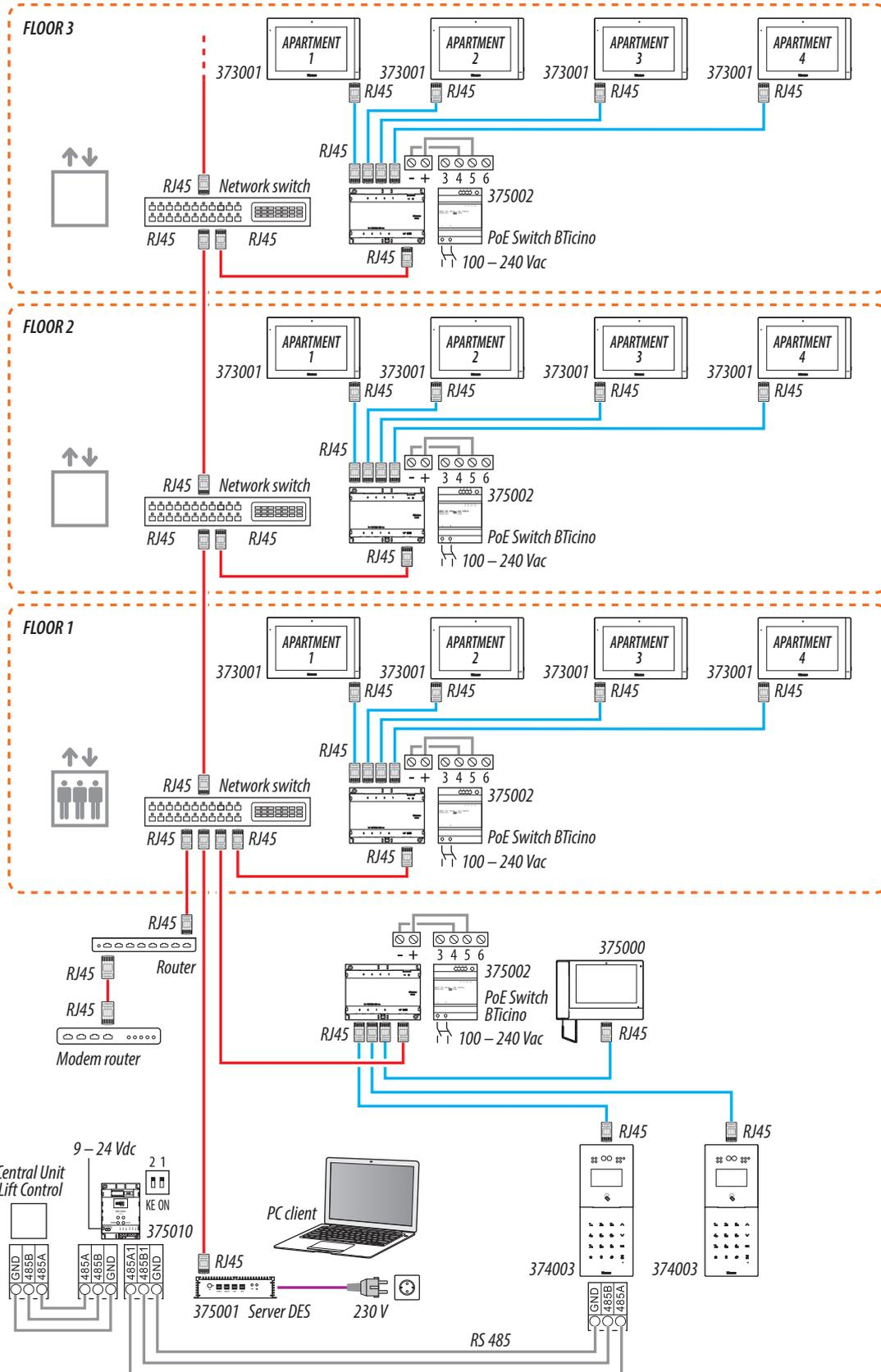
**Attention:** do not directly connect PoE ports to an unsuitable network interface, such as a device powered by a different voltage. Connect the UP LINK port to a suitable port, never to a PoE port.
