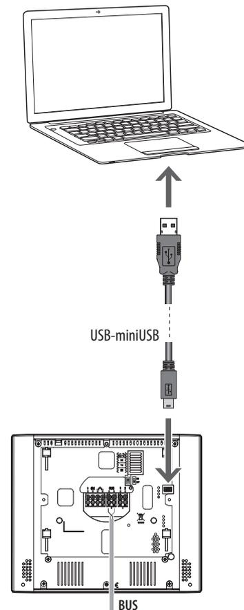
To ensure that the communication is successful, the video internal unit must be powered.
