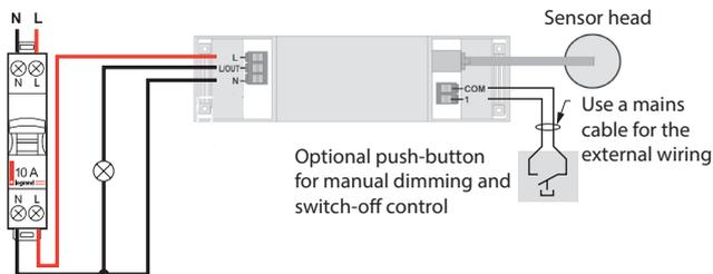
**⚠** The maximum cable length between the sensor head and the power unit is 1 metre
