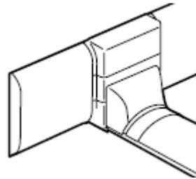
For branching from skirting-trunking 80/120x20 mm to floor duct
