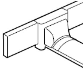
For branching from mini-trunking 60x20/75x20 mm to floor duct
