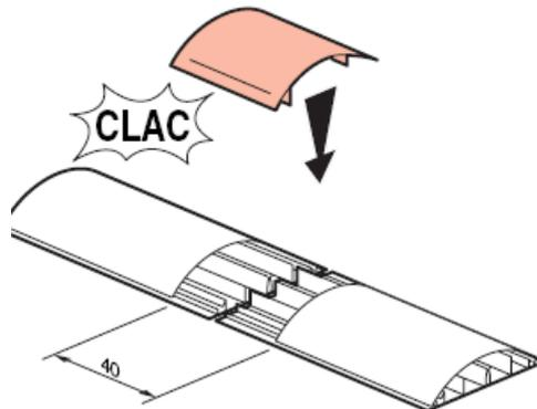
For mounting with floor ducts 92x20mm
