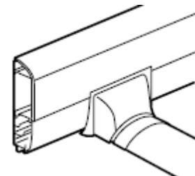
For branching from skirting-trunking 140x35 mm to floor duct
