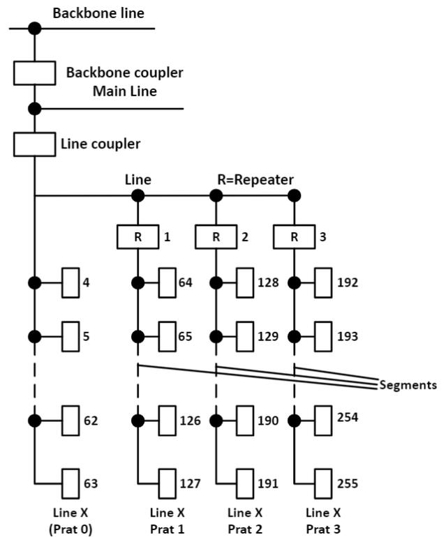
Fig.1 Connection of repeaters to a bus line
