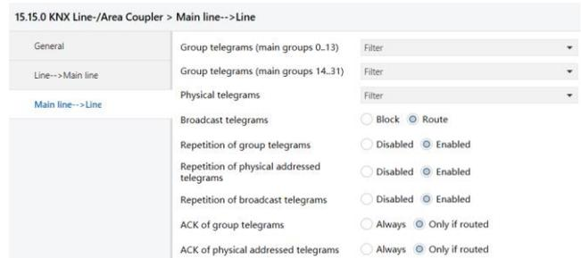
Fig.5.1.3 Parameter window “Main line-->Line”
