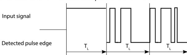
Once a pulse edge has been detected at the input, further edges are ignored for the duration of the debounce time TD. The process of preventing debounce in the below chapters are the same with here. TD is the effective time of a pulse edge input, namely the period after a input signal is recognised as a operation.
