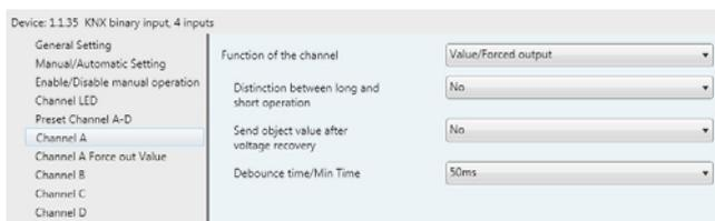
Fig.7.11(2) Parameter window "Value / Force output, X" (No distinction long/short operation)
