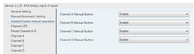
Fig.7.3 Parameter window "Enable/Disable manual operation"
