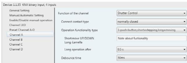
Fig.7.16 Parameter window "Shutter control, X"
