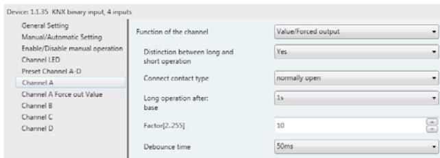
Fig.7.11(1) Parameter window "Value / Force output, X" (Distinction long/short operation)
