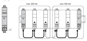
Note: in a system (beneath an Nemo SX/Modbus interface) it is possible to use a maximum of 3 power supply modules = 3 groups of 500 mA.
