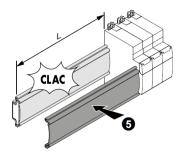
Clip the protection plastic cover on the remaining exposed part of the communicating rail
