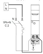
. Power supply protected by a Fuse holder:
