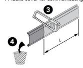
Cut the protection plastic cover to the required length
