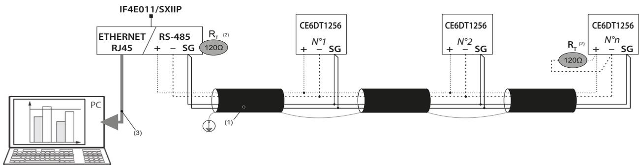
(1) RS485: Required use of Belden 9842, Belden 3106A (or equivalent) for a maximum length of 1000 m, or Category 6 cable (FTP or UTP) for a maximum length 50 m
