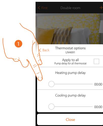
1. Touch to set a delay time for the activation of the pumps thus avoiding them starting before the zone valves have opened, both for heating and cooling.
