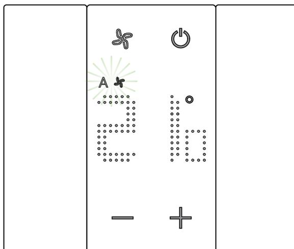
During the adjustment the fan symbol and the segment for the speed selected flash. After a few seconds, the value is saved and the symbol shows the new adjustment.
