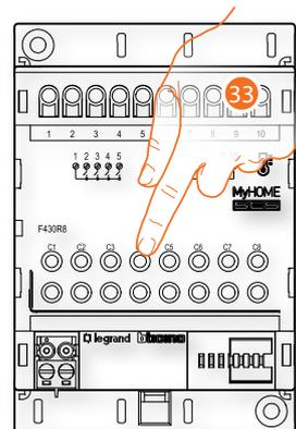
33. Touch any one of the pushbuttons on the actuator on the system
