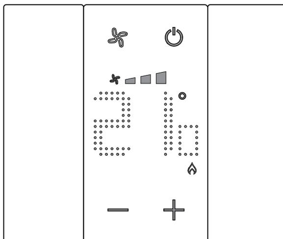
After a few seconds, the new setting is saved and the measured temperature appears. This example shows a set temperature higher than the measured temperature, therefore also displaying the symbol confirming that the heating system is in operation 🔥.
