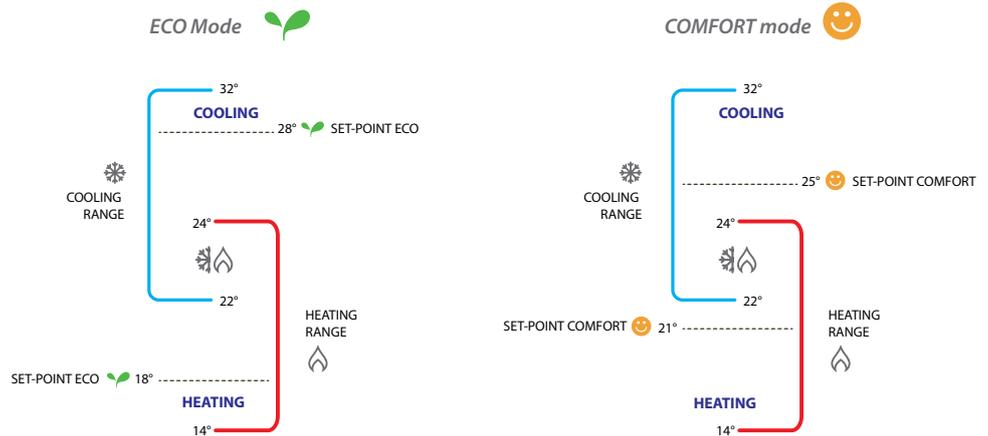
The above example indicates the temperature set-point pairs for Eco mode and Comfort mode.
