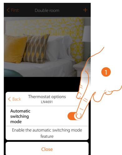
1. In systems with 4-pipe fancoils enabled for both heating and cooling or in systems where the water circulation systems for heating and cooling are completely independent, you can enable this function to manage the switching between heating and cooling automatically.
