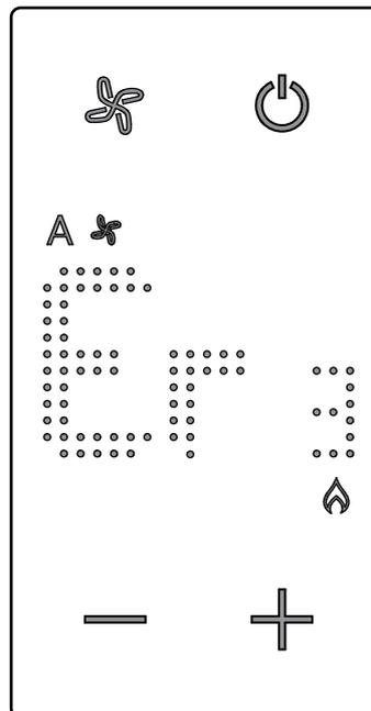
**\*Note:** if ER4 or a temperature significantly different from the one perceived are displayed, or after the first installation, wait at least 5 hours before checking the operation again and completing the calibration procedure.
