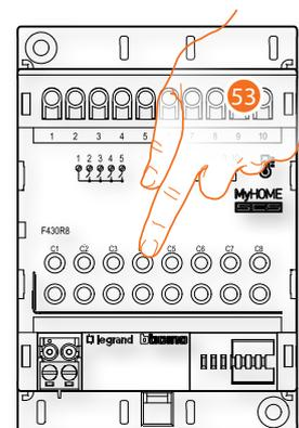
53. Touch any one of the pushbuttons on the actuator on the system
