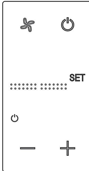
When the thermostat is OFF, this symbol appears. The OFF command can only be sent using the Hotelsupervision software, or the local window contact.
