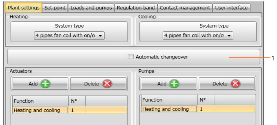
1. **Automatic change:** in systems with 4-pipe fancoils enabled for both heating and cooling or in systems where the water circulation systems for heating and cooling are completely independent, you can enable this function to manage the switching between heating and cooling automatically.
