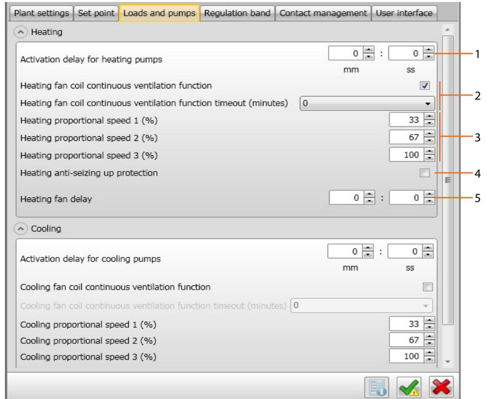
1. **Delay pump activation:** you can set a delay time for the activation of the pumps thus avoiding them starting before the zone valves have opened.
