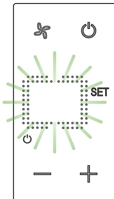
This symbol flashing quickly indicates that the thermostat has not yet been configured
