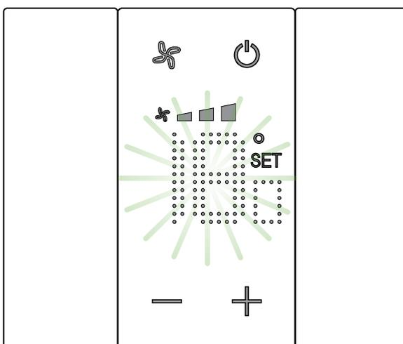
The display shows the **SET** symbol and the currently programmed temperature. If this value is acceptable, wait for flashing to end. The temperature will not be changed.
