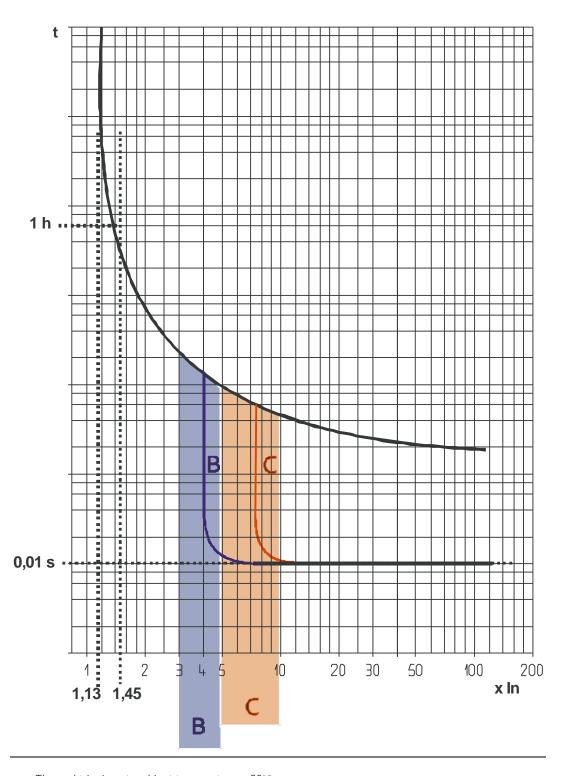
Thermal tripping at ambient temperature =  $30^{\circ}$ C In = circuit breaker rated current
