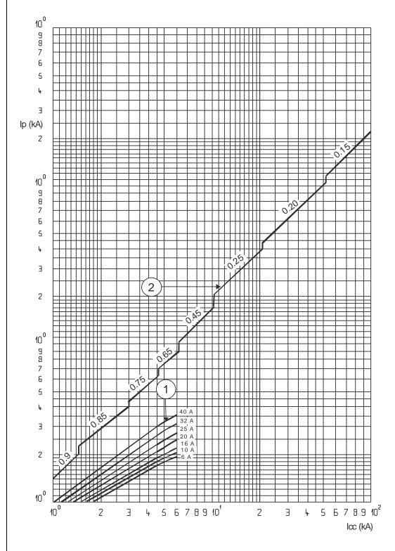
lcc = Prospective short-circuit symmetrical current (rms value in kA)
