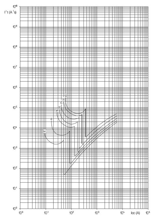
lcc = prospective short-circuit symmetrical current (rms value in A)  $I^2t$  = limited thermal stress (in A s) $^2$
