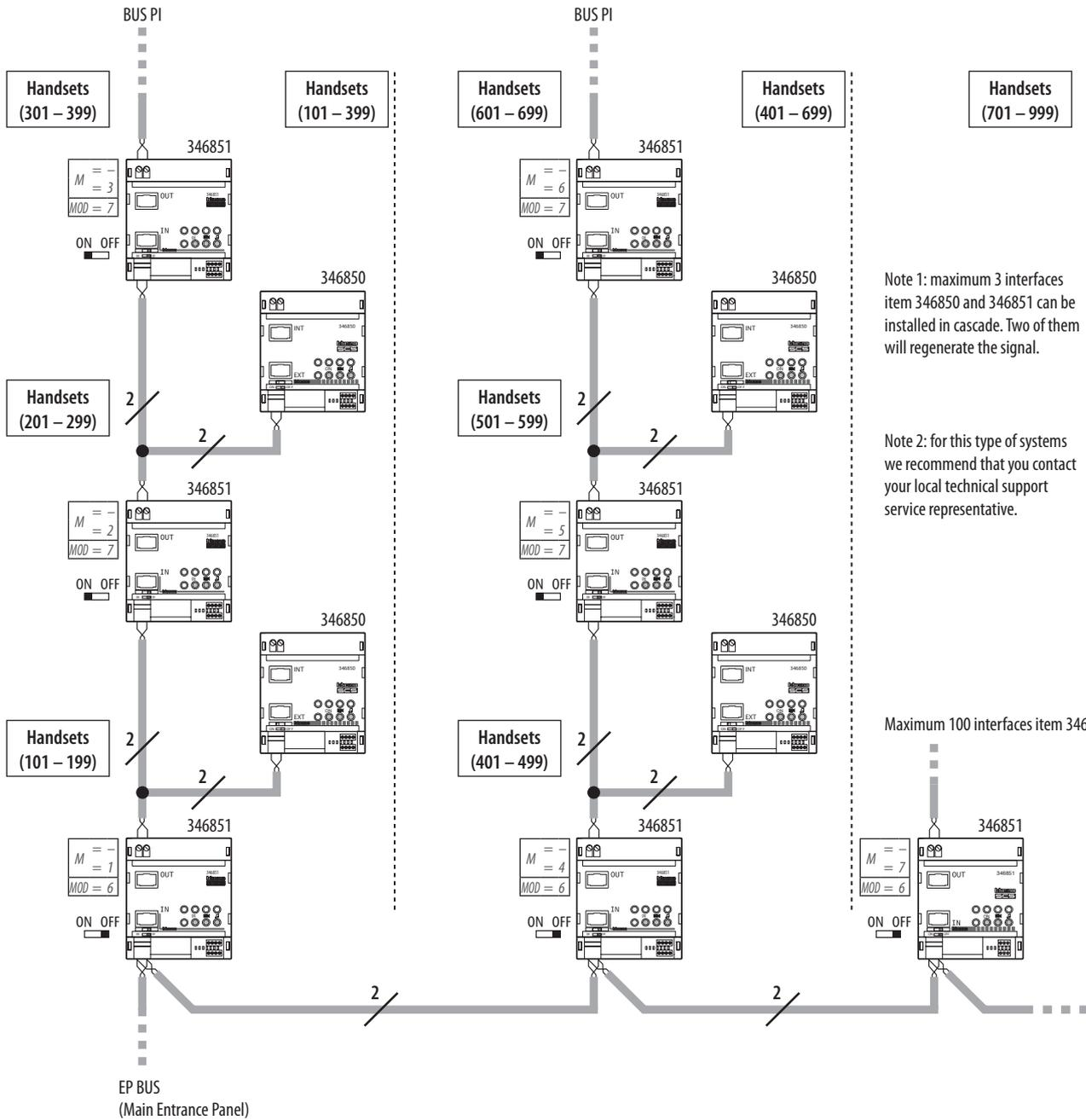
Note 1: maximum 3 interfaces item 346850 and 346851 can be installed in cascade. Two of them will regenerate the signal.
