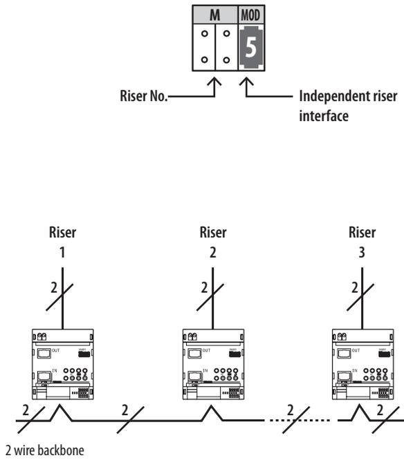
The handsets connected to the single riser will be identified at the main entrance panel by the M configurator of 346851 x 100 + the N configurator of the single handset.
