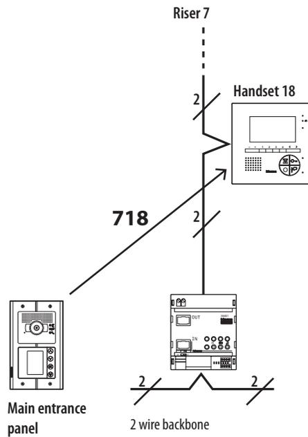
As far as the EP is concerned, the handset is number 718: this is the M of 346851 (7) x 100 + N of the handset connected to the riser (18).
