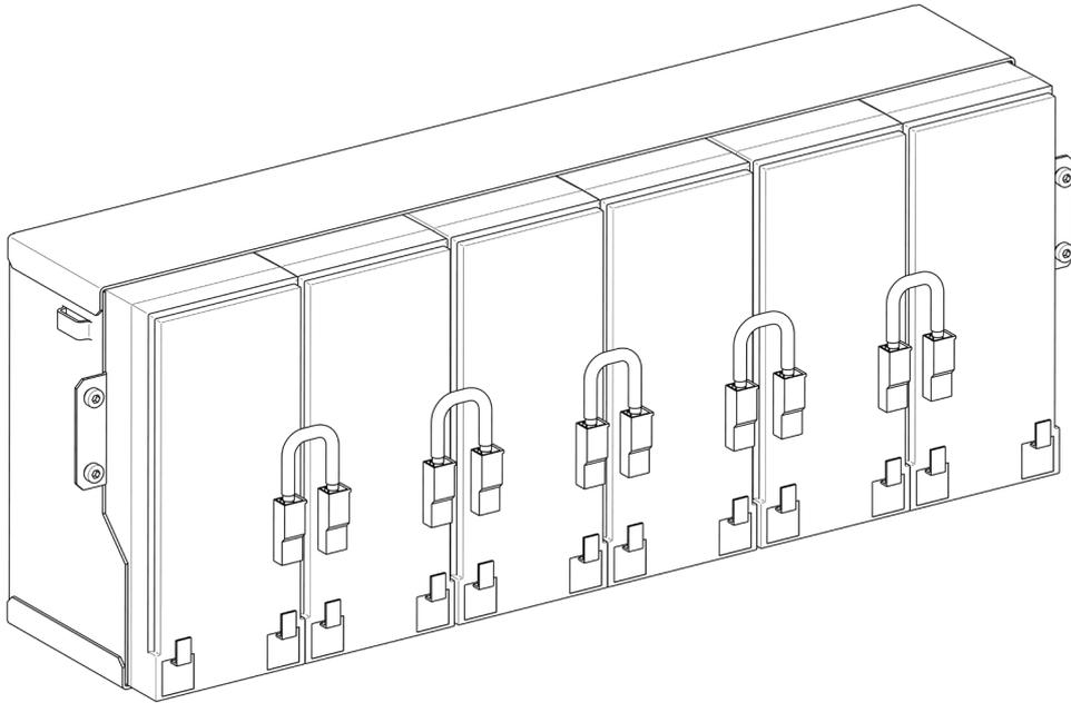
Keep the batteries firm to the block by fixing a metal bar with the four screws provided.
