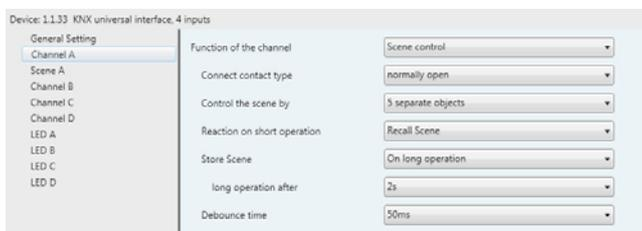
Fig. 8 Parameter window "Scene control, X"
