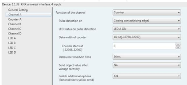
Fig.12 Parameter window "Counter, X"
