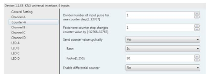
Fig.13 Parameter window "Counter-X"
