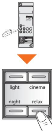
In the Scenario Module press the programming enabling pushbutton.
