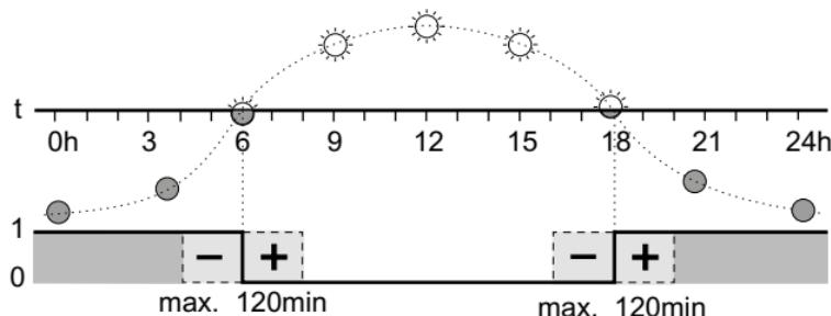
The time switch switches on at the calculated sunset time and off at the calculated sunrise time.
