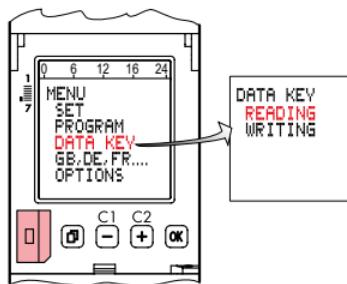
**Load the programs from the data key to the time switch (READ KEY)**
