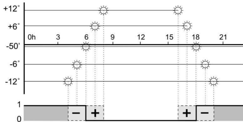
If the offset setting is in degrees the time switch switches on and off at times of equal brightness, despite the differences in twilight time lengths over the course of the year.
