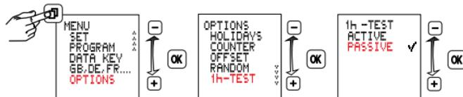
After one hour, the time switch returns automatically to the programmed mode.
