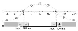
The time switch switches on at the calculated sunset time and off at the calculated sunrise time.
