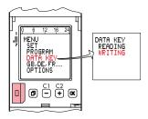
Load the programs of the time switch on to a data key (WRITE KEY) Warning! all programs stored on the data key will be overwritten.
