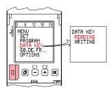
Load the programs from the data key to the time switch (READ KEY) Warning! all programs programmed in the time switch will be overwritten.
