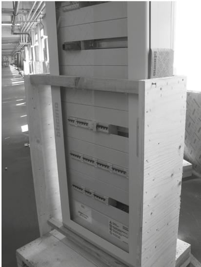
Fig. 2 - Panel shipped vertically on a pallet
