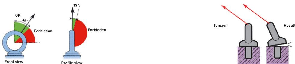
In the case of slinging on several rings, the following regulations must be observed:
