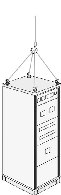
Fig. 3A - Lifting the panels with cables
