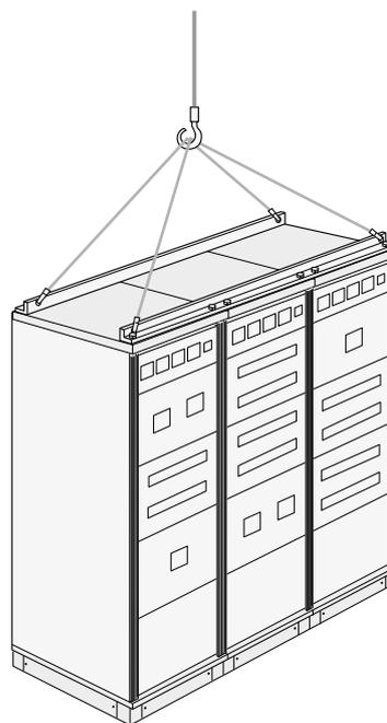
Fig. 3B - Lifting the panels with cables and angle crossbars. (this assembly is to be done by the panel builder under his responsibility)
