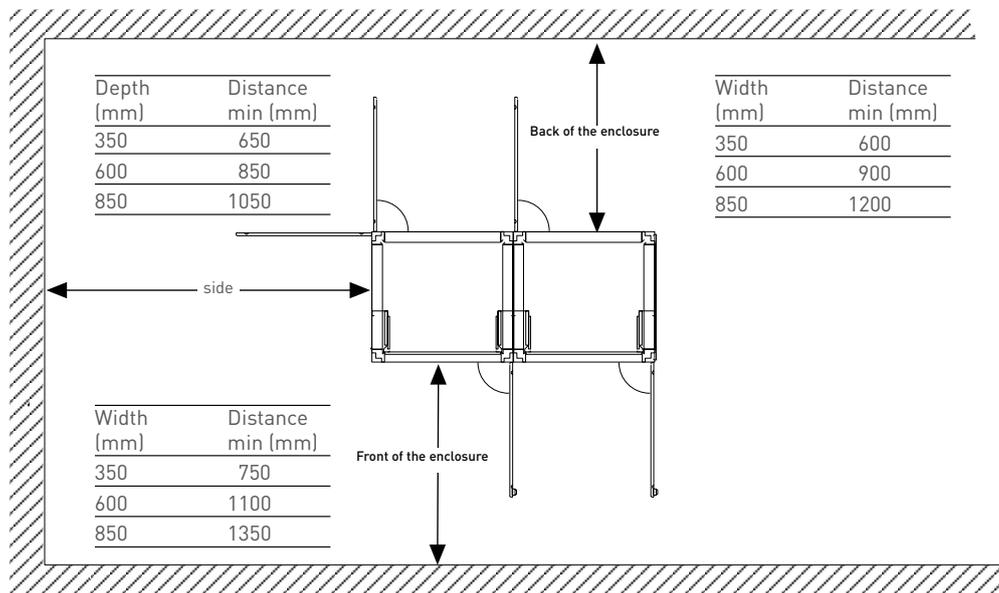
Fig. 4 - Recommended minimum clearances between panel and walls
