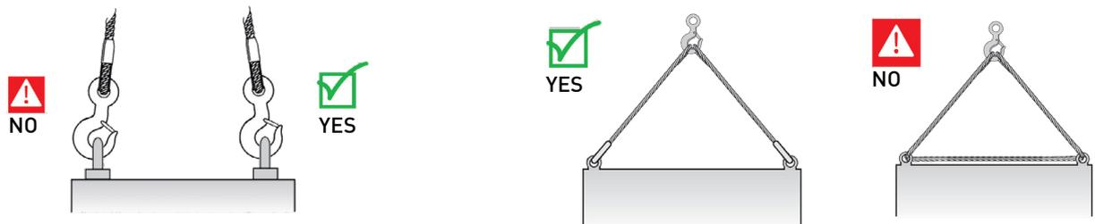
During the lifting operation, the angle formed by the sling and the ring must be respected:
