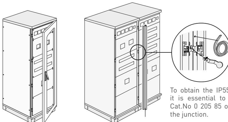
To obtain the IP55 degree of protection, it is essential to insert the sealing kit Cat.No 0 205 85 on the whole surface of the junction.
