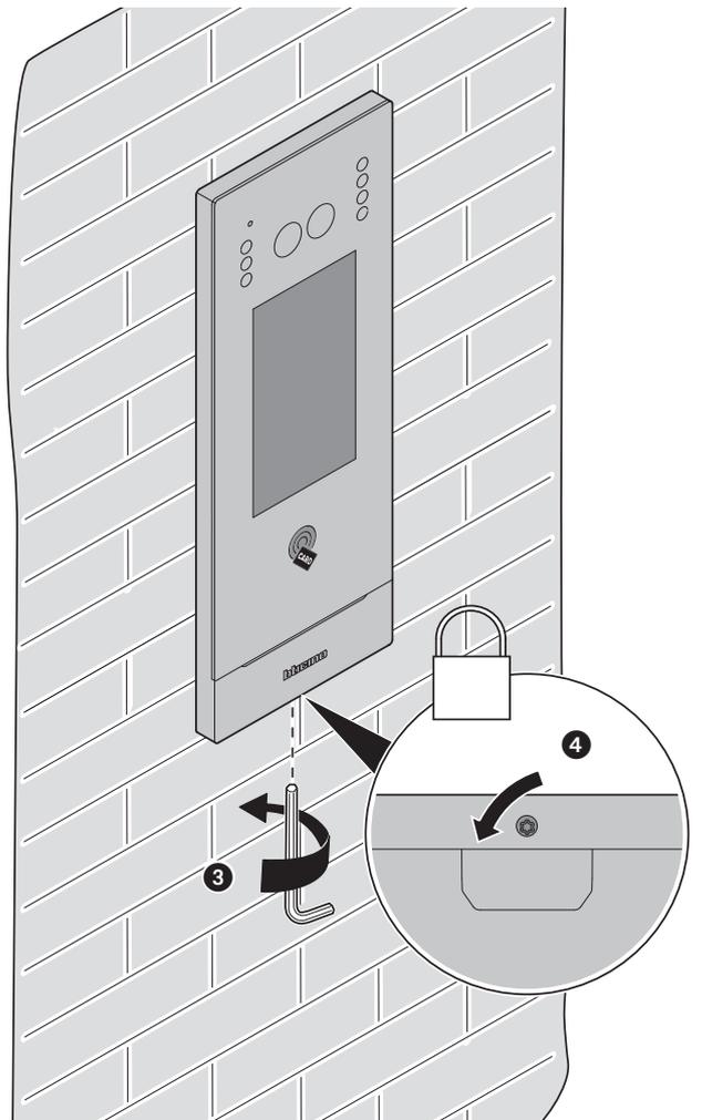
\* Adjust the tamper screw so that it presses the tamper switch of the device and activates the anti-theft function in case of removal sending an alarm to the guard station.
