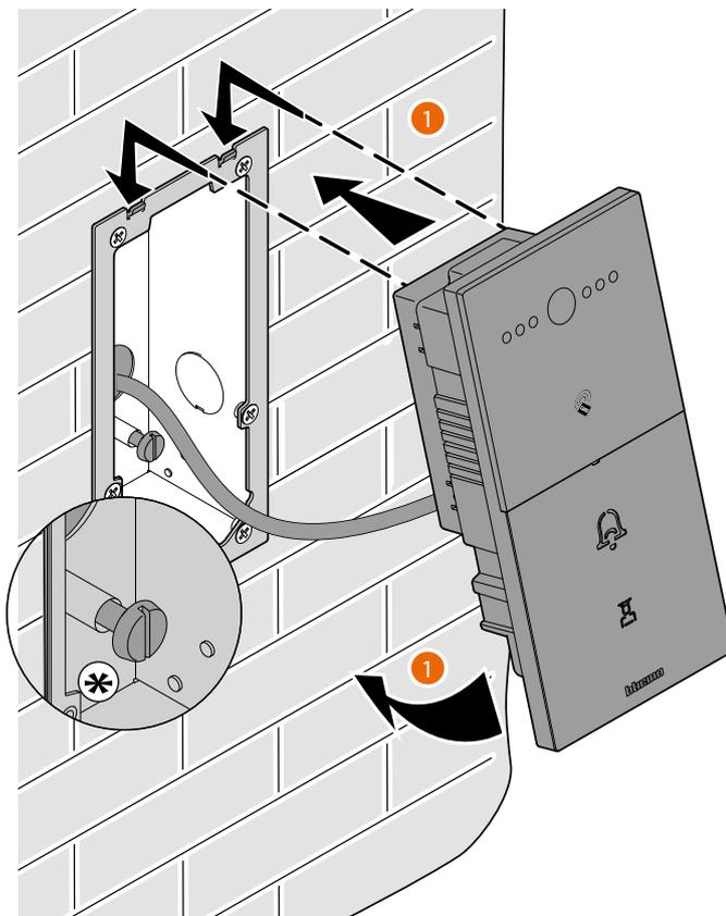
(\*) Adjust the tamper screw so that it presses the tamper switch of the device and activates the anti-theft function in case of removal sending an alarm to the GS.
