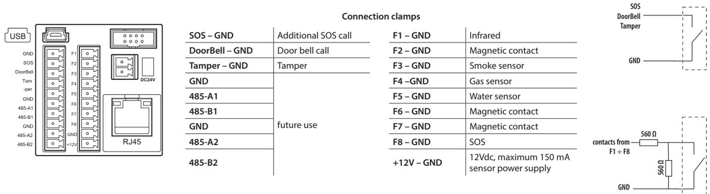
All contacts must be connected to GND and the corresponding dedicated input. The functions and wiring mode of the inputs are set by default as shown in the table and diagram, they can be customized using the software and/or straight from the device. Tamper and Doorbell input are not customizable and SOS-GND is disable by default.
