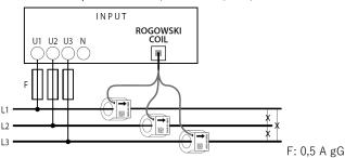
4 wires three-phase network, 3 sensors (3N-3E):
