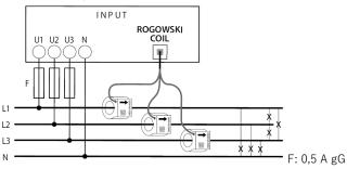
. Rogowski coil(s) cable length (see § Overall Dimensions) allow you to put Nemo SX Measure modules everywhere in the installation. This is not mandatory to have them near to the associated protection device of the measured line.
