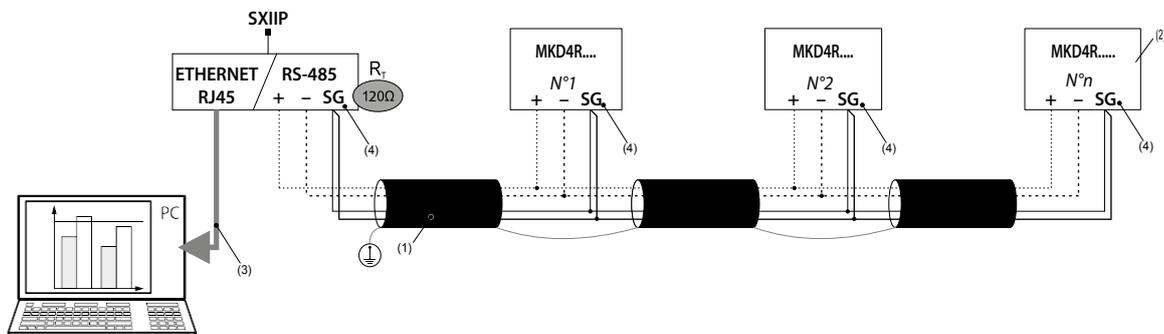
(1) BELDEN 9842, BELDEN 3106A (or/equivalent) max. 1000 m, Cat. 6 (FTP/UTP) max. 50 m
