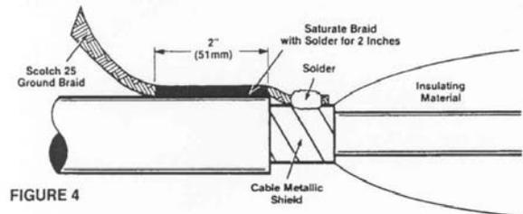
When grounding termination or joints: Solder Scotch 25 Ground Braid to cable metallic shields and bring remainder of braid out of joint or termination. Construct a 51mm solder block on ground braid to prevent moisture penetration into joint.
